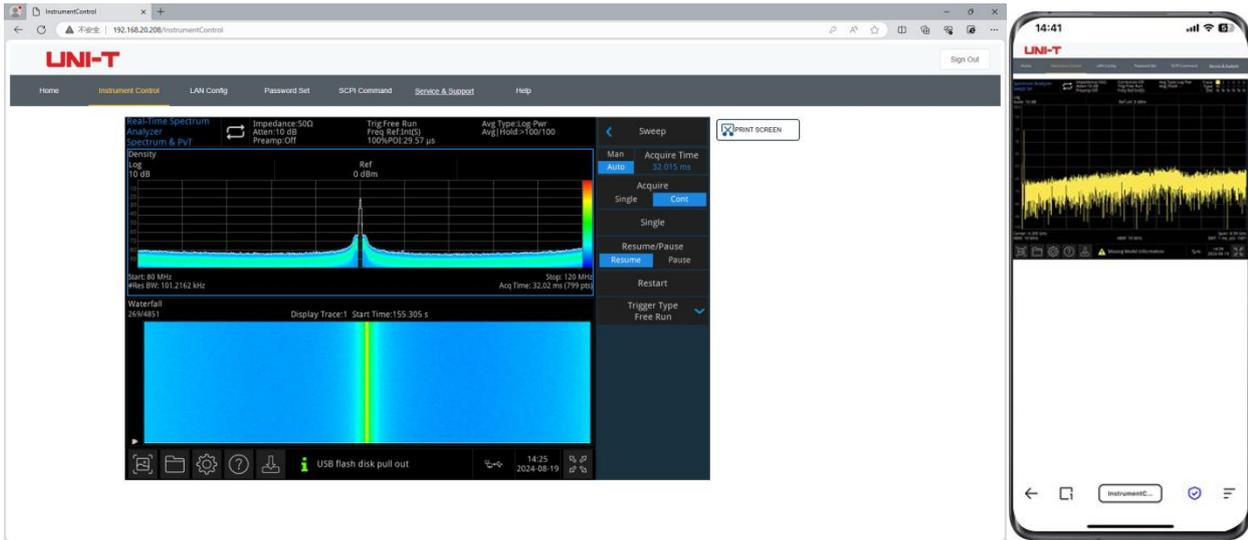
Supports SCPI remote control, remote viewing, and control of exported trace data, as well as other operations. It enables online browsing and use and supports access from both PCs and mobile phones.
