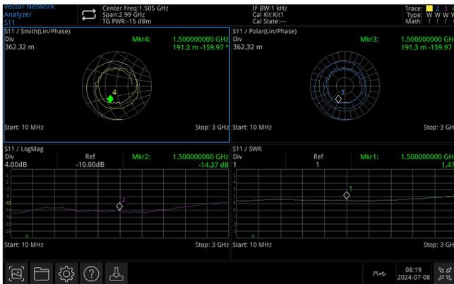
VNA mode allows for precise characterization of the network properties of measured components and circuit networks by measuring S11 and S21 parameters, with various display methods such as Smith charts and polar coordinates. The touch to based interface simplifies the measurement process, enabling users to achieve better results in less time.
