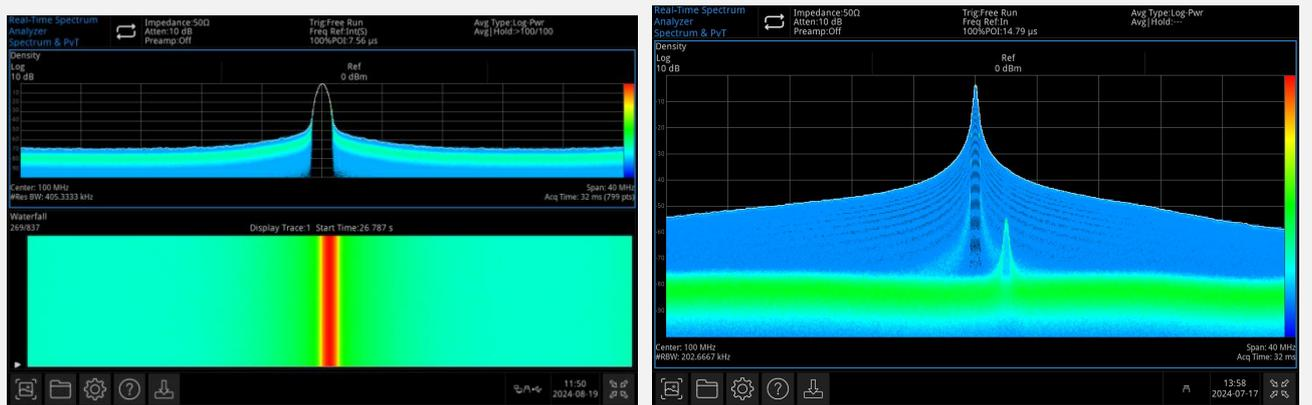
Use combined display with density spectrograms for continuous spectral display, visualizing the frequency occurrence of signals and capturing small signals in the presence of larger ones
