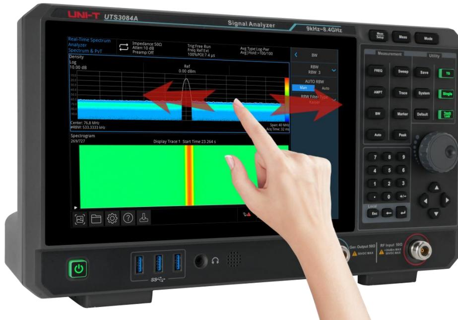
The 10.1-inch multi-touch HD capacitive screen offers quick menu settings and supports various gestures, including dragging, expanding, and zooming on traces. This user-friendly interface enhances human-to-computer interaction, addressing issues of cumbersome and complex operations.
