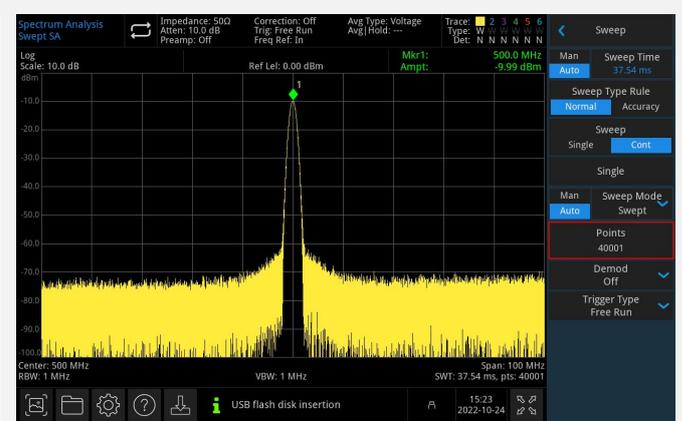
UTS3000A series provides up to 40,001 sweep points, offering higher frequency resolution and making it easier to capture hard-detect signals.
