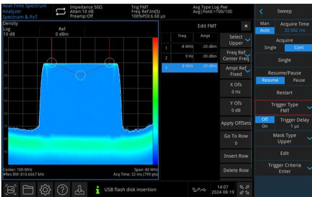
Use the frequency template trigger to generate the measurement of episodic or transient signals.
