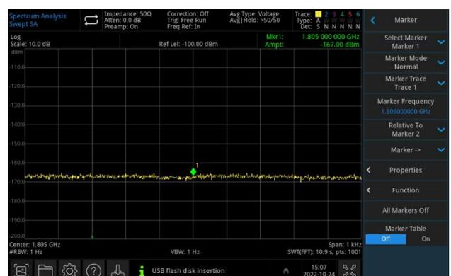
Weak signal testing can be significantly impacted by the noise floor of the spectrum analyzer. With a DANL as low as -165 dBm, UTS3000A series provides excellent sensitivity, enabling effective testing of weak signals.
