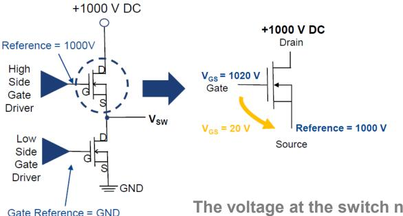
The voltage at the switch node ( $V_{SW}$ ) swings between the supply voltage (1000V) and the low-side reference voltage (GND).
