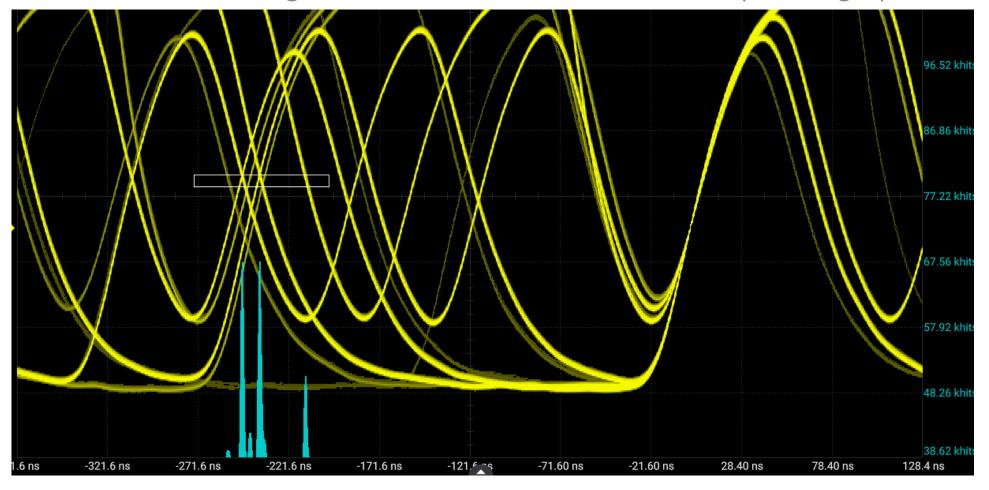
2) mask test – can be used to check that digital bus signals have the correct shape and comply to the standard defined voltage/time boundaries
