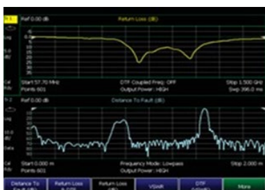
View return loss and DTF simultaneously
