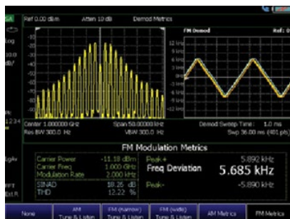
Characterize AM/FM signals using AM/FM demodulation
