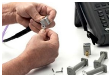
Easily use waveguides with FieldFox
