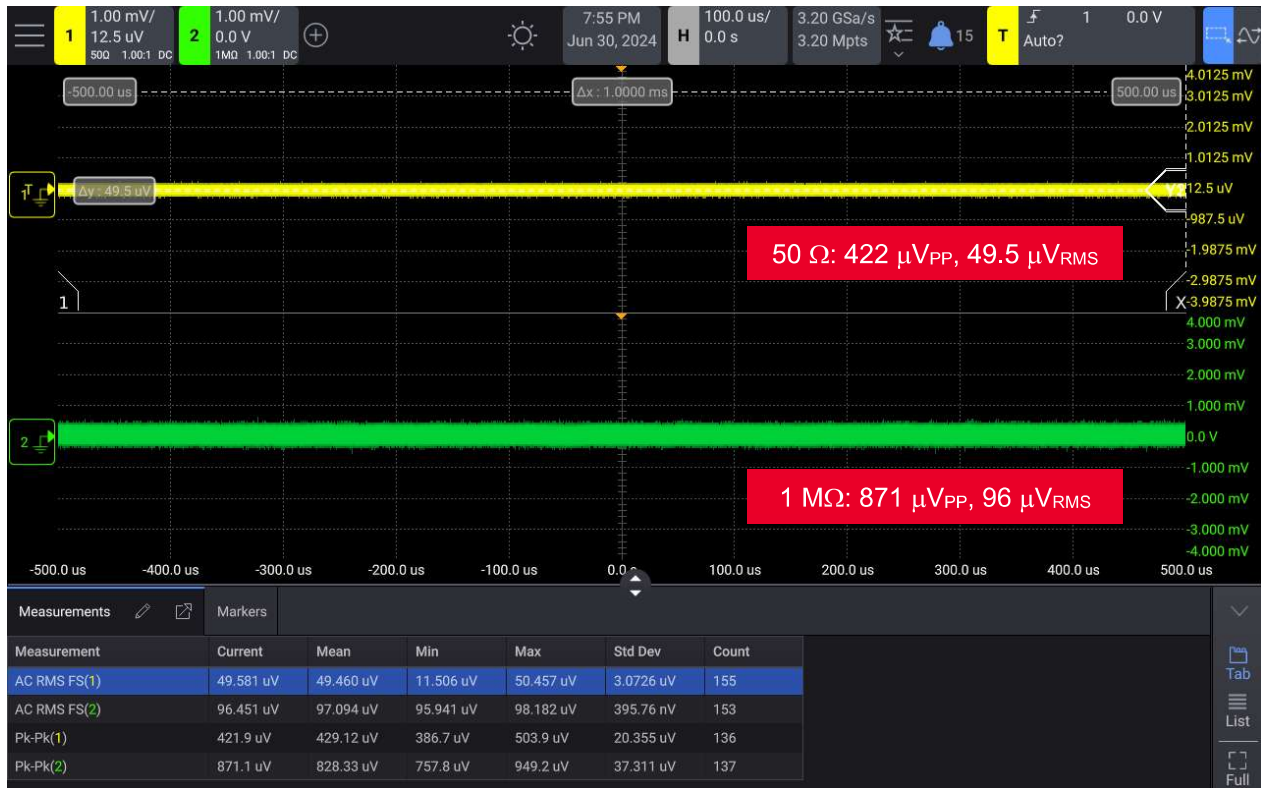
Figure 4. Baseline noise on the 50 Ω input compared to the 1 MΩ input path of the HD3 oscilloscope
