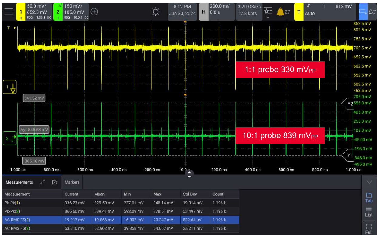
Figure 3. Noise comparison of a 1:1 and 10:1 probe measuring the output ripple on a power supply
